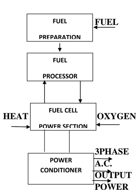
**Schematic of a fuel cell power plant**
