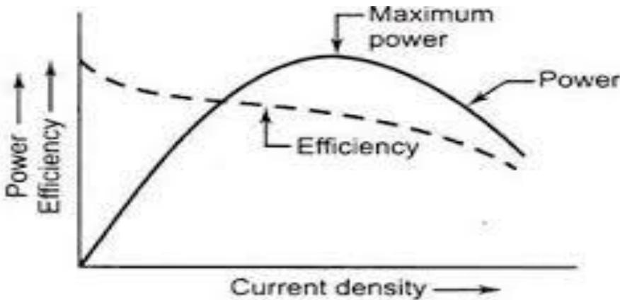
Power and efficiency characteristics of a fuel cell.
