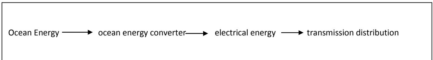
With off shore energy conversion plants the energy transmission from off shore energy conversion plant to land based load center is in the form of HVDC submarine cable transmission.
