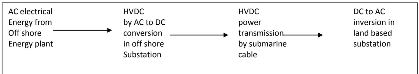
With on shore ocean energy, conversion plant, the costly HVDC conversion substations are avoided. The energy route is simpler:
