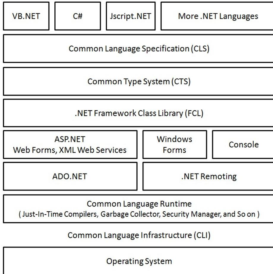
**Figure 1** An overview of the .NET architecture.
