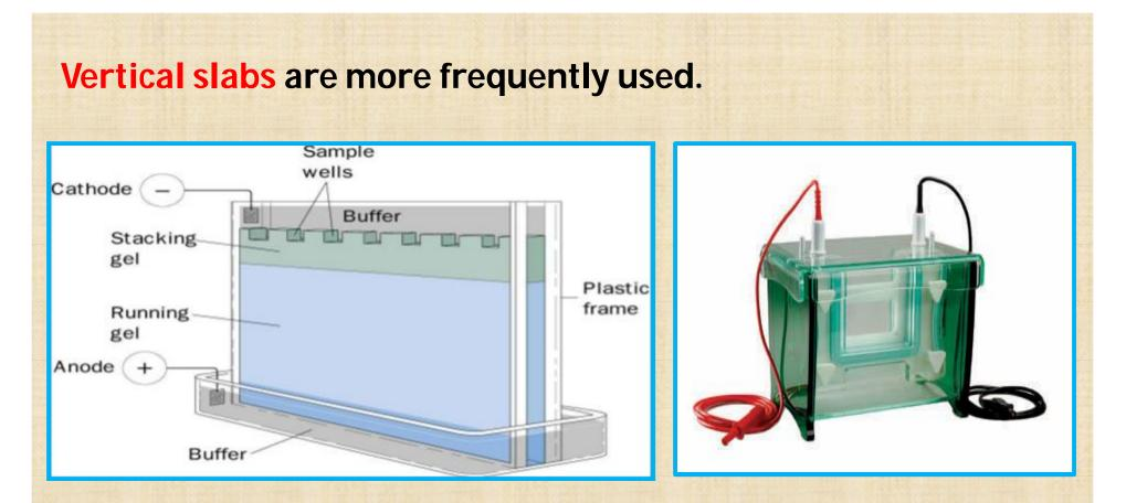
Slabs of gel carry more samples (up to 25 samples can be run on a single gel plate) making them more economical to use and enabling more samples to be compared with each other when run under identical conditions.
