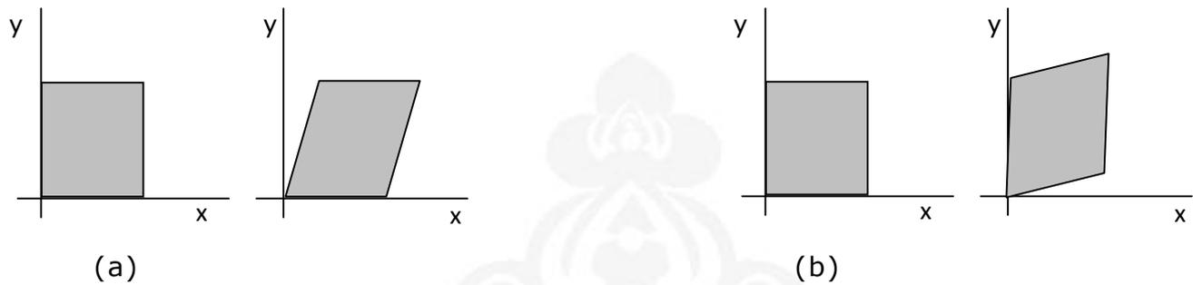
An object after (a) x-direction shear and (b) y-direction shear
